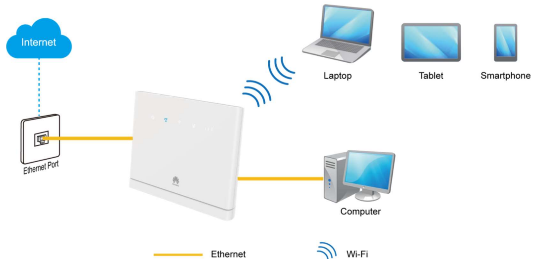
Figure 4-2 Accessing the Internet through an Ethernet network
